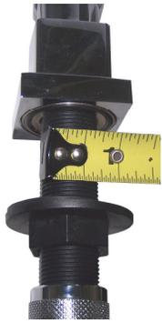
Before drilling the counter, measure the threaded part to avoid making a too large hole.
