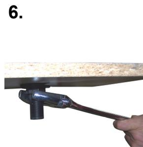
With a wrench, tighten the black fixing nut. Please do not use excessive force.
