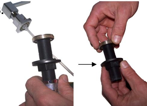
Unscrew the bottle, the black fixing nut and removed the rubber gasket
