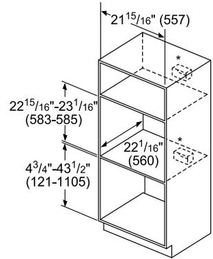
\* For wall installations, the junction box may be located above or below the unit within reach of the power cable.
