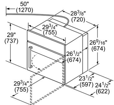
Allow 3/4" (19 mm) gap to nearest cabinet face for door swing on SideOpening models
