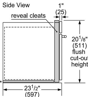
\* Flush installation requires a  $\frac{5}{16}$ " (8 mm) high x  $28\frac{1}{2}$ " (724 mm) wide x  $22\frac{1}{2}$ " (571 mm) deep baseplate underneath the unit body.
