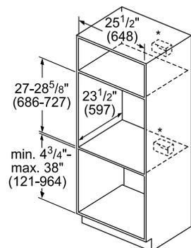
\* For single ovens installed into a wall cabinet, the junction box may be located above or beneath the unit within reach of the power conduit.
