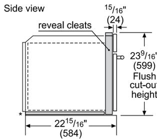
\* Flush installation requires a 3/16" (5 mm) high x 21 15/16" (557 mm) wide x 22 1/16" (560 mm) deep baseplate underneath the unit body.
