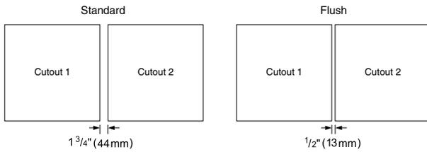
The ovens will overlap the cutout resulting in a 1/2" (13mm) spacing between the products
