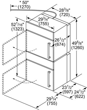
\*\* Allow 3/4" (19 mm) gap to nearest cabinet face for door swing on SideOpening models
