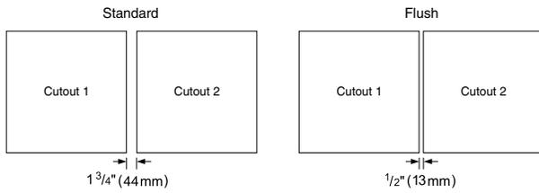
SideOpening Door Models: If another product is installed adjacent to the side hinge we recommend to increase each distance by an additional 1/4" (6mm) to leave room for the door to open and close freely.
