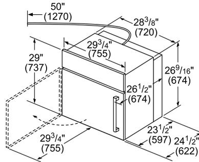
Allow 3/4" (19 mm) gap to nearest cabinet face for door swing on SideOpening models
