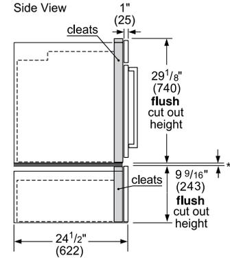
\*IMPORTANT: base has to be able to support oven weight. Please check oven manual for minimum weight requirements.
