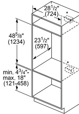
\* Junction box may be installed above, below, or to the left or right of the unit within range of the power conduit.
