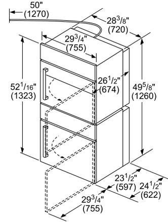
\*\* Allow 3/4" (19 mm) gap to nearest cabinet face for door swing on SideOpening models
