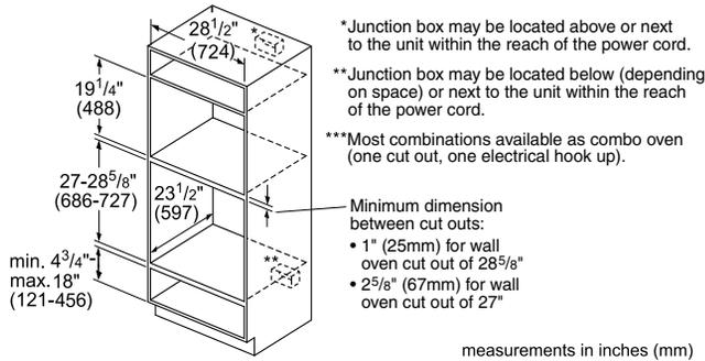
NOTE: This configuration is available as a combo oven (one cut out, one electrical hook up) – HBL5751UC (500 series) and HBL8751UC (800 series)
